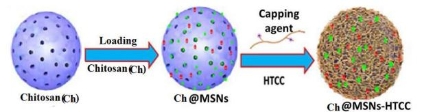
**Fig. 1:** An illustration of the loading process of chitosan onto mesoporous silica nanoparticles as well as the creation of Ch@MSNPs20nm-HTCC.
